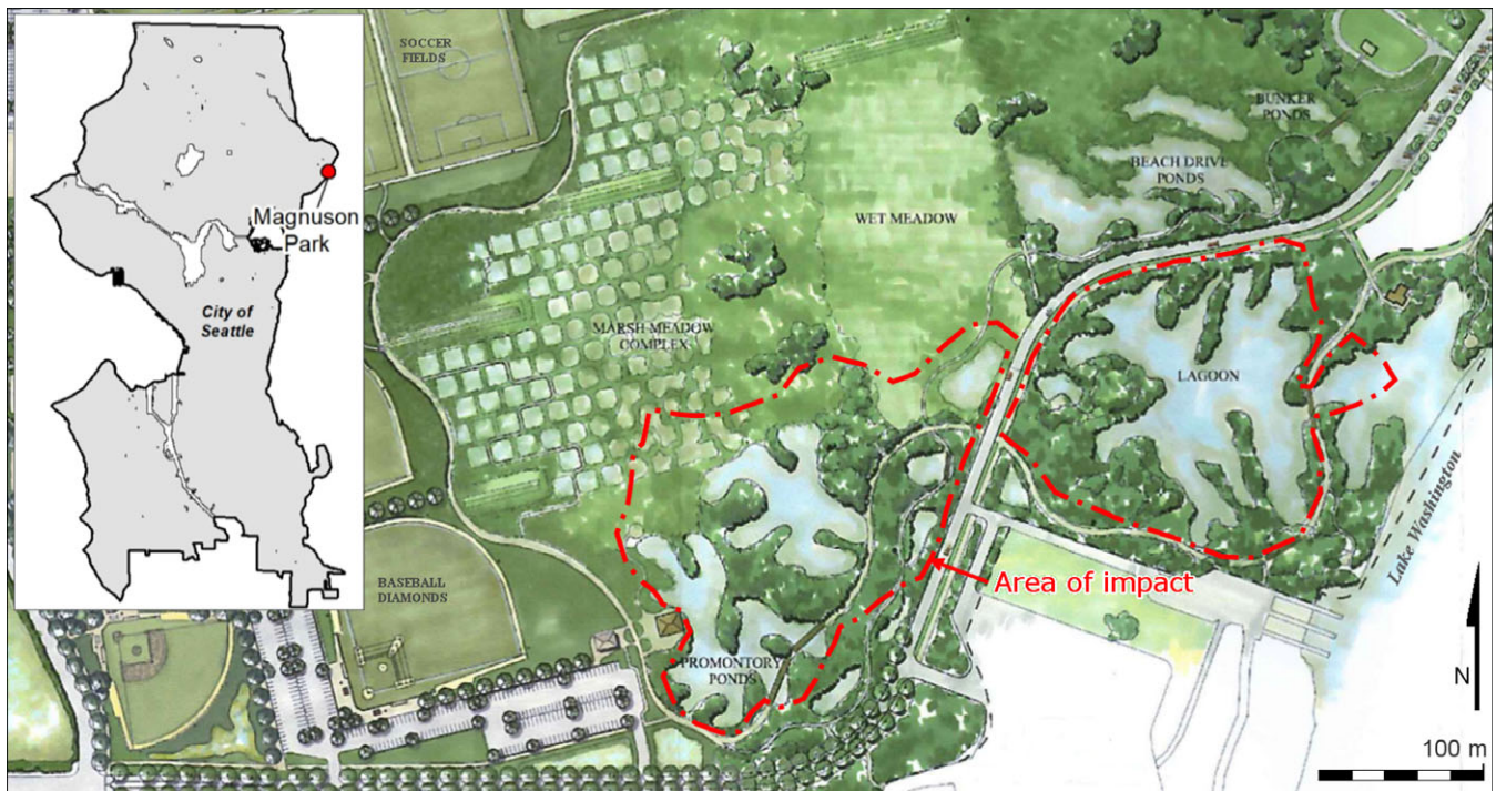
FIGURE 4 Design plan for the Magnuson Park wetland complex, Seattle, WA. Completed in 2012, it includes a variety of water features including large ponds, wetland, and nonperennial vernal pools. Beaver colonized in 2014 and created additional ponding area within the areas originally designed to be wet meadows and vernal pools. Original design plans, adapted from the Berger Partnership (Seattle, WA, USA)
